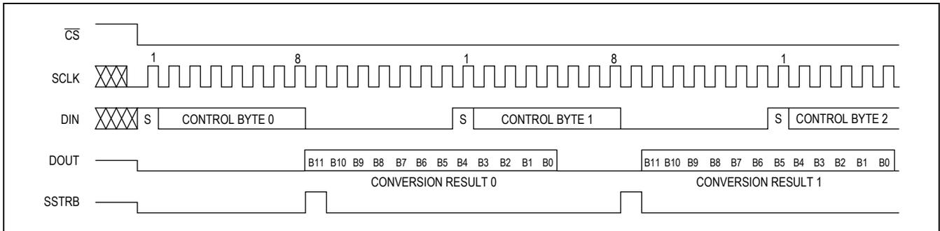
Figure 11a. External Clock Mode, 15 Clocks/Conversion Timing
