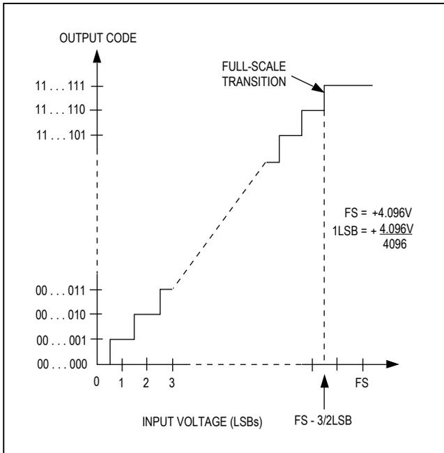
Figure 15. Unipolar Transfer Function, 4.096V = Full Scale
