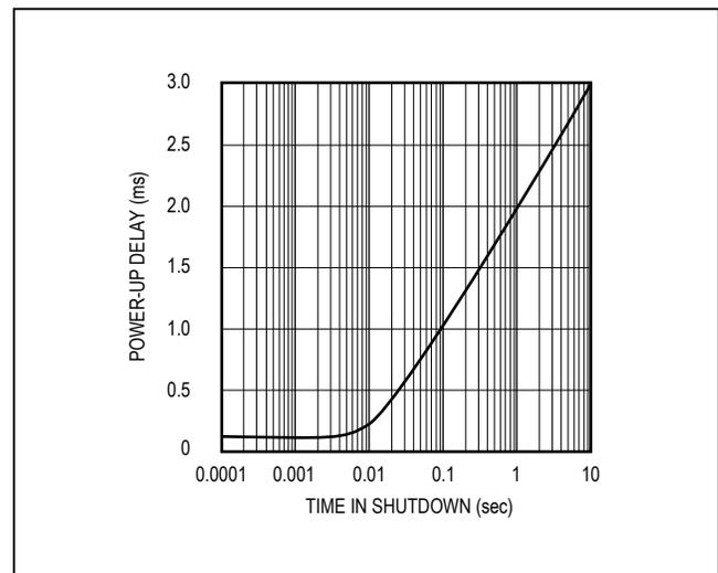
Figure 14c. Typical Power-Up Delay vs. Time in Shutdown
