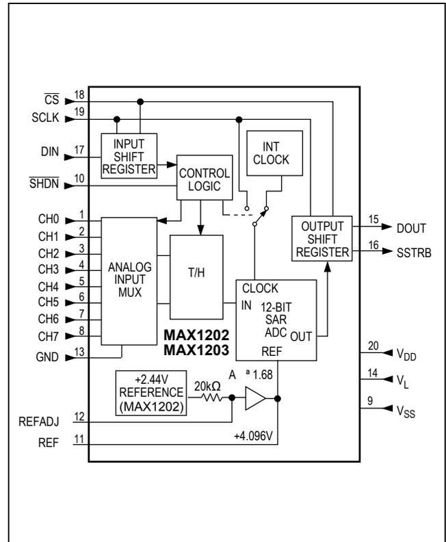
Figure 3. Block Diagram
