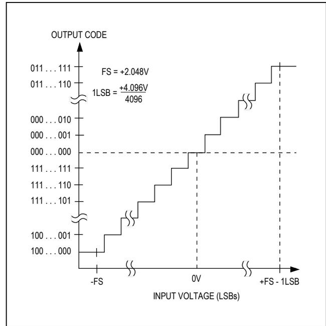
Figure 16. Bipolar Transfer Function, ±4.096V/2 = Full Scale
